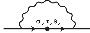
FIG. 3. Feynman diagram describing the renormalization of the SO potential by the Coulomb interaction. The solid line represents the electron propagator and the wavy line is the Coulomb interaction.
