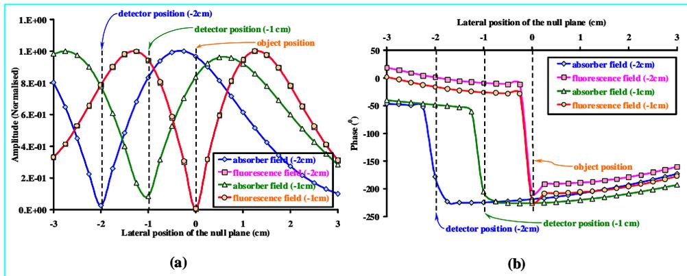
**Fig. 7:** Profile of the simulated field, (a) amplitude (b) phase for a scanning of the two sources and two positions of the detector. Due to the normalization, the two amplitudes of the fluorescence fields overlap.
