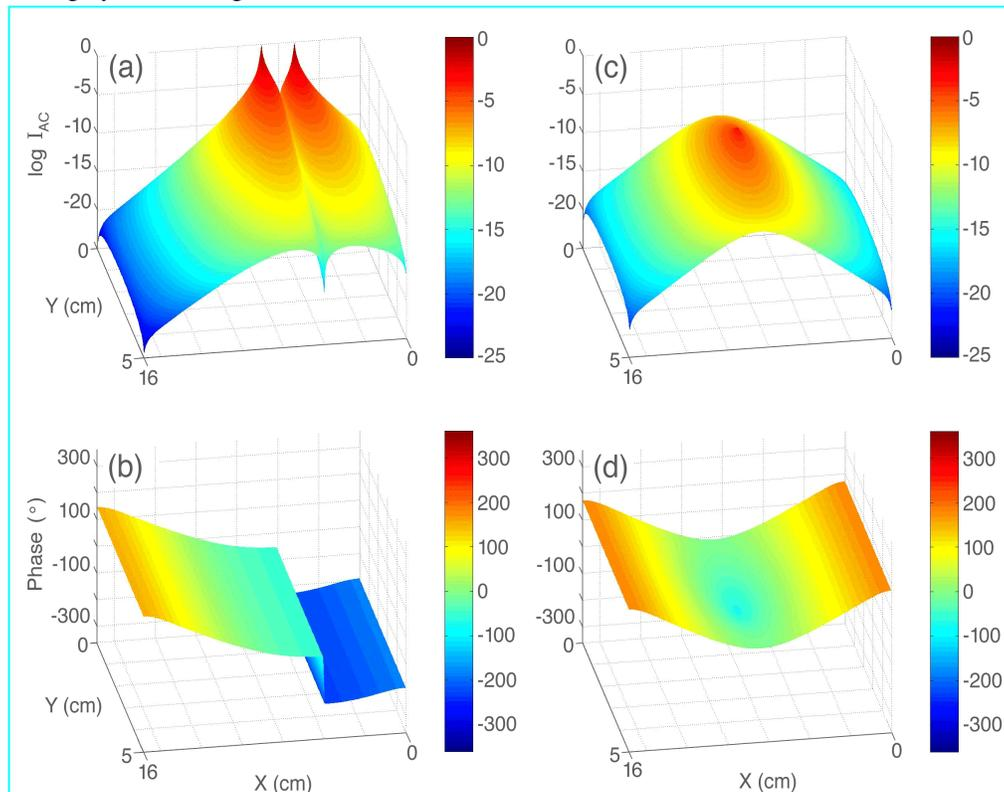
**Fig. 3:** (1.5 MB) Movie of (a) logarithm of the amplitude at the excitation wavelength – (b) phase at the excitation wavelength – (c) logarithm of the amplitude at the fluorescent wavelength and (d) phase at the fluorescent wavelength. The object is located in the center of the media (maximum of re-emitted amplitude). The sources plane correspond to the  $y=0$  plane and the detectors plane correspond to  $y=5\text{cm}$  plane.
