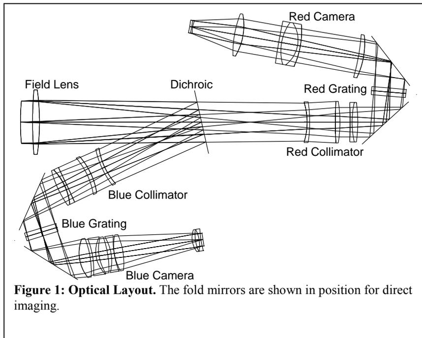
Figure 1 is an optical layout of the spectrograph. The field lens is located 60 mm beyond the focal plane to minimize the impact of defects. Immediately following the field lens, a dichroic mirror directs the red (transmitted) and blue (reflected) light into two separate optical paths. A pair of flat mirrors tunes the VPH gratings while maintaining Littrow condition, as described below. It will be possible to use gratings with resolution up to  $R = 11,000$  for a 1 arcsec slit.
