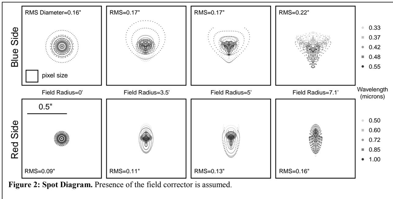
**Figure 2: Spot Diagram.** Presence of the field corrector is assumed.
