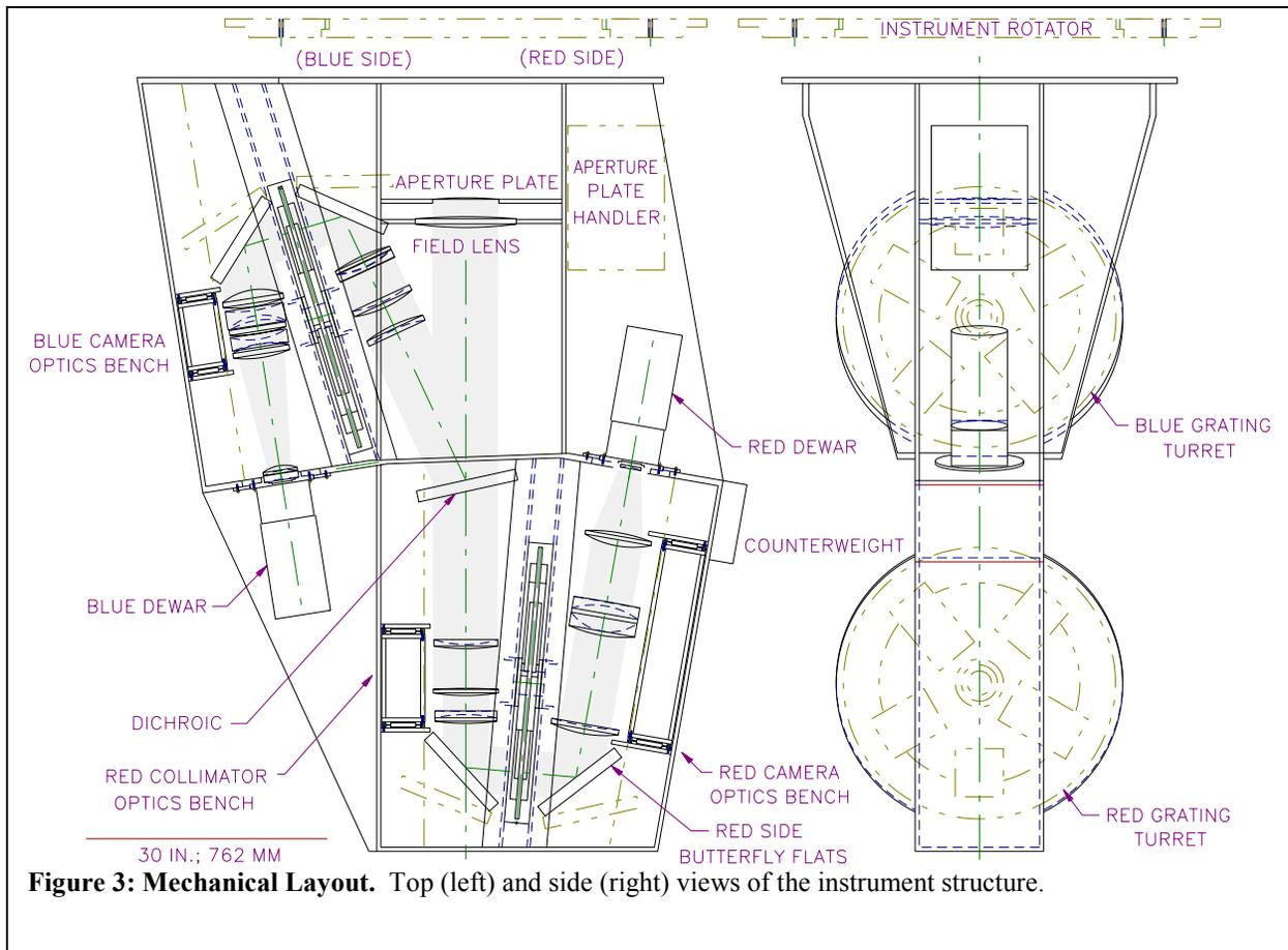
A finite element analysis of the preliminary design, which includes realistic local deflections for individual optics mounts, indicates that the design goals are achievable with this structure. A similar structure is being used to construct the *MIKE* spectrograph.
