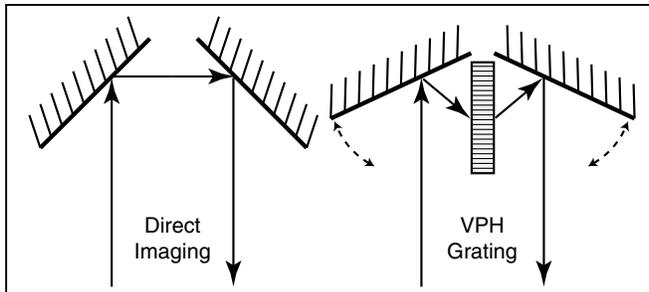
**Figure 4: “Butterfly Mirror” Mount for VPH Gratings.** A symmetric rotation of the two fold mirrors takes the incoming and outgoing beams from a direct imaging configuration (left) to a high-dispersion mode through a VPH grating (right). Smaller mirror motions tune the spectrograph wavelength. With grating fringes perpendicular to the surface, as shown, the butterfly mirror guarantees that the spectrograph is in Littrow and at the peak of the blaze function.
